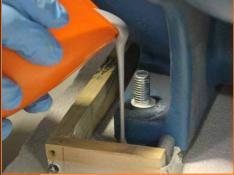
Belzona 7111 can be poured easily without the need of additional resin and the risk of particles settling prior to its cure time.
