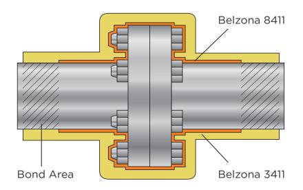
The Belzona flange protection system is a combination of two products.
