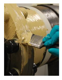
Belzona 3411 can be easily applied by brush and it does not require heat or specialist tools for its application.
