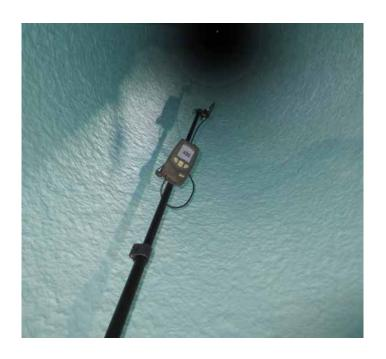
Belzona 1523 provides long-term corrosion and chemical resistance to equipment operating in continuous immersion at temperatures up to 140°C (284°F). This spray-applied coating has a 24-hour overcoat window which allows large projects to be effectively and quickly completed, reducing downtime dramatically.
